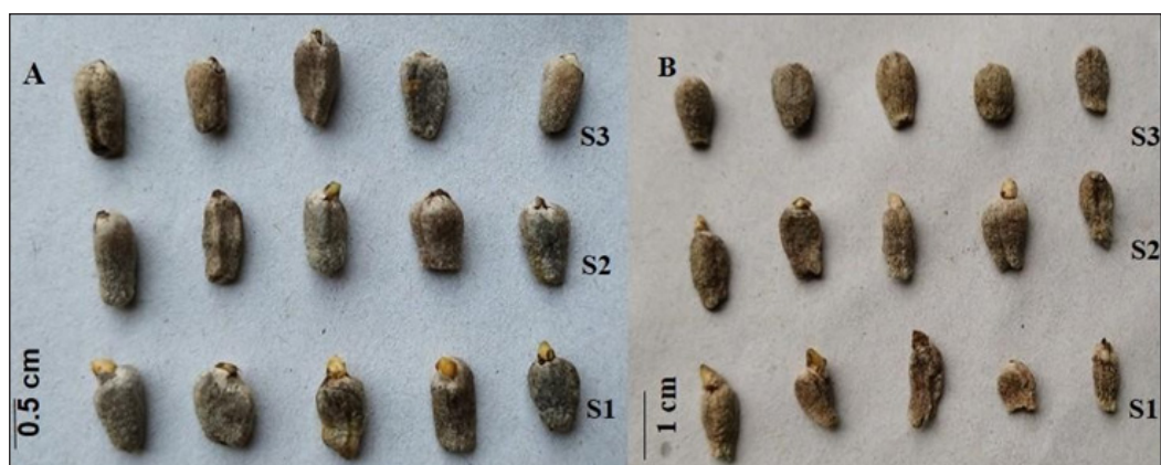
Figure 4. Seed appearance after a month (A) and five months (B) storage of S1 (27-32°C, >60% RH); S2 (20-23 °C, 50-60% RH); S3 (5-7 °C, 40-50% RH)
